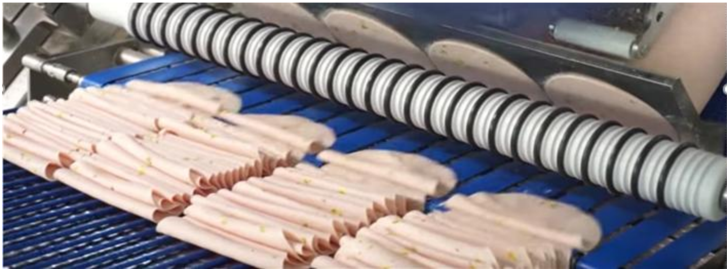
Slicer with portioning folder
