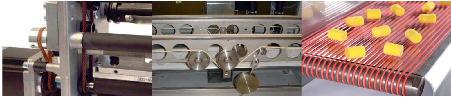
Vulkollan round belt in a label printer
