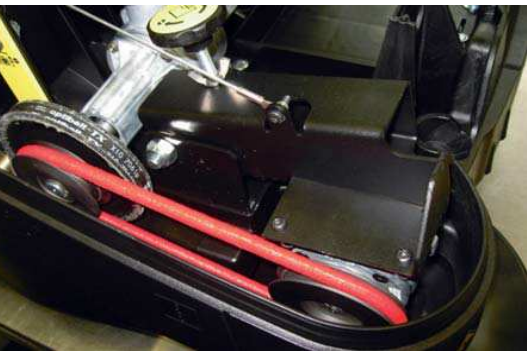
Endless elastic round belt, PU red inside the engine compartment of a cleaning machine
