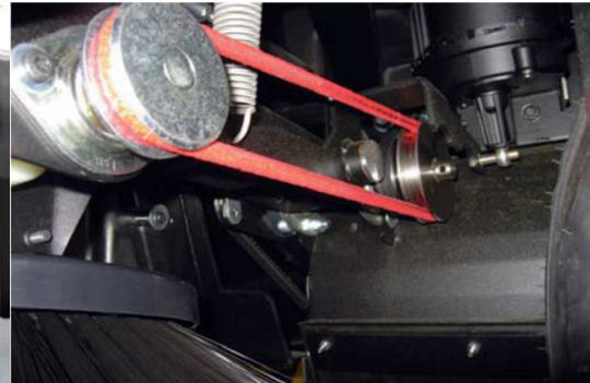
Lateral broom drive of a power sweeper
