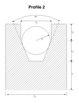
b1 = Ø + 10% b 2 = Ø + 80% h1 = 80% from Ø h2 =  $\frac{1}{2}$ Ø r =  $\frac{1}{2}$ Ø d = Pulley - Ø
