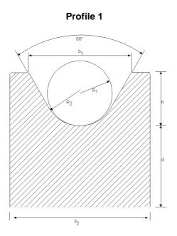
b1 = Ø + 55,6 % b2 = 2 x Ø h = 80% from Ø r1 =  $\frac{1}{2}$  Ø r2 =  $\frac{1}{2}$  Ø + 10% d = Pulley - Ø
